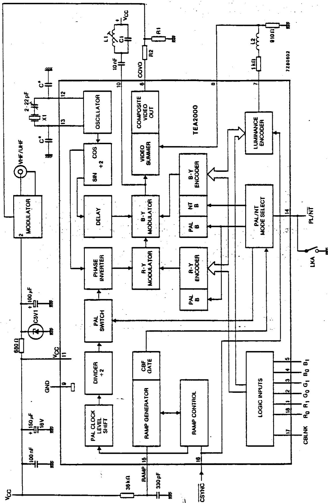
Fig. 2 Internal circuit details and typical external connections.
